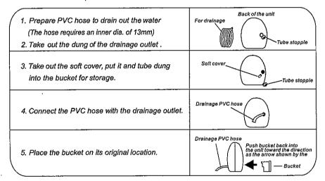
The Proper Way To Place The Water Drainage PVC Hose When using continuous drainage, the PVC hose most be placed below the drainage hole.
