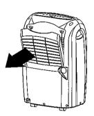
B. Clean the filter by using a vacuum cleaner or washing it with clean water. Then dry the filter with a cloth.
